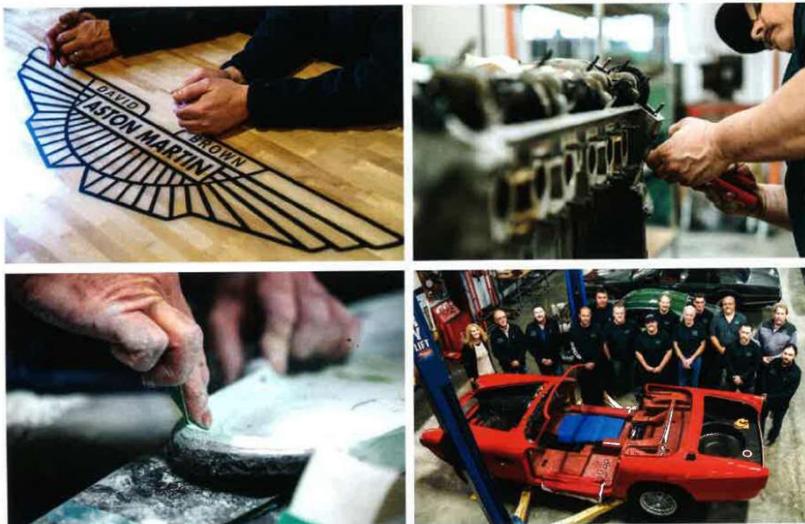
Clockwise from above Body prep, painting and finishing can take up to 900 man-hours per car; DB-era Astons have become the backbone of KKR's business; reassembling a classic straight-six in the engine shop; and that 14-strong workforce in full
